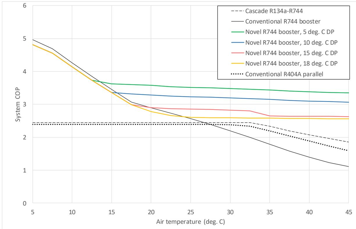
Fig. 1 Overall system COP for a constant low temperature and medium temperature load of 50 kW and 150 kW, respectively. For air temperatures below the dew point temperature, dew points are assumed equal to the air temperature (saturated air condition).
