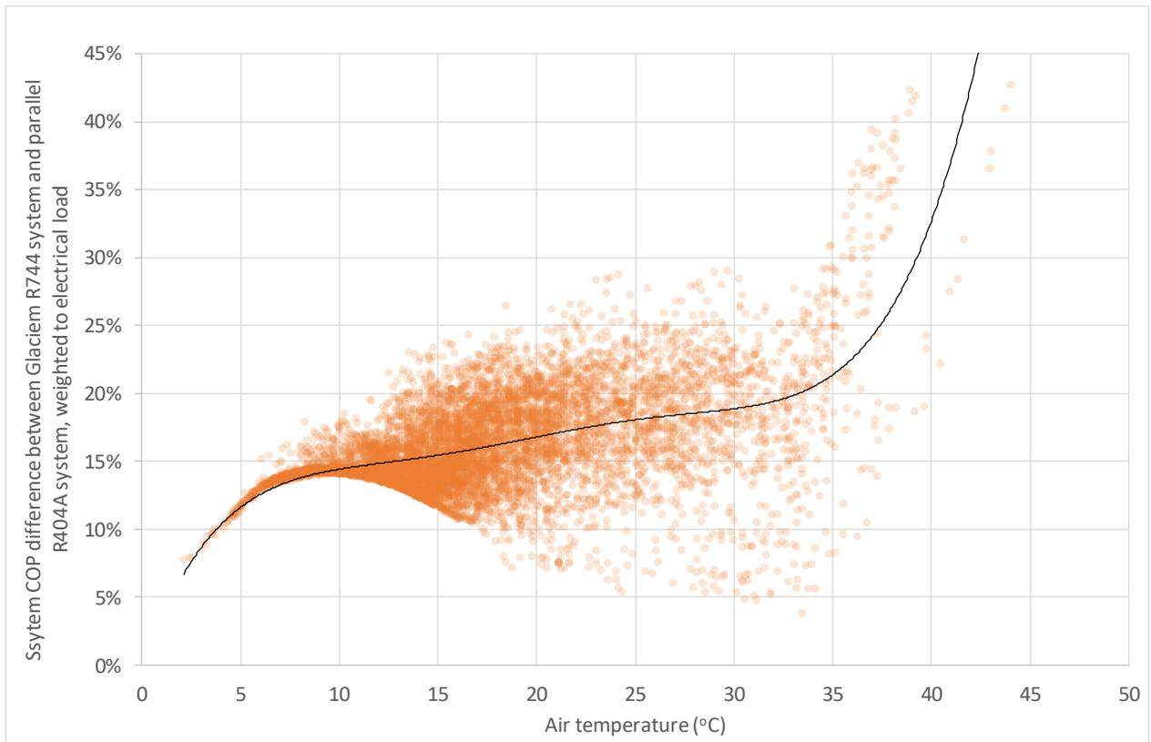
Fig. 3 Relative improvement in system COP between the novel R744 system and conventional parallel R404A system for each hour of the year, weighted against the electrical load.
