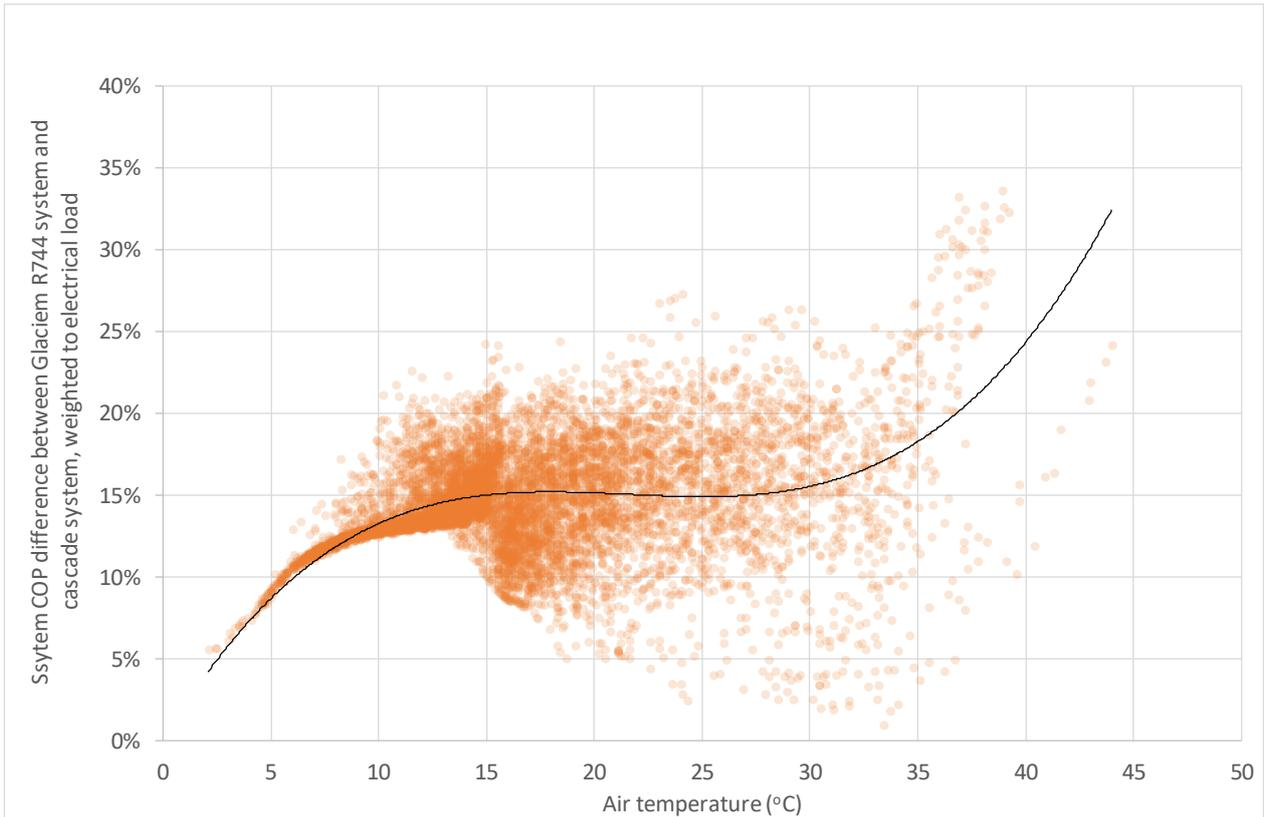
Fig. 2 Relative improvement in system COP between the novel R744 system and cascade system for each hour of the year, weighted against the electrical load.
